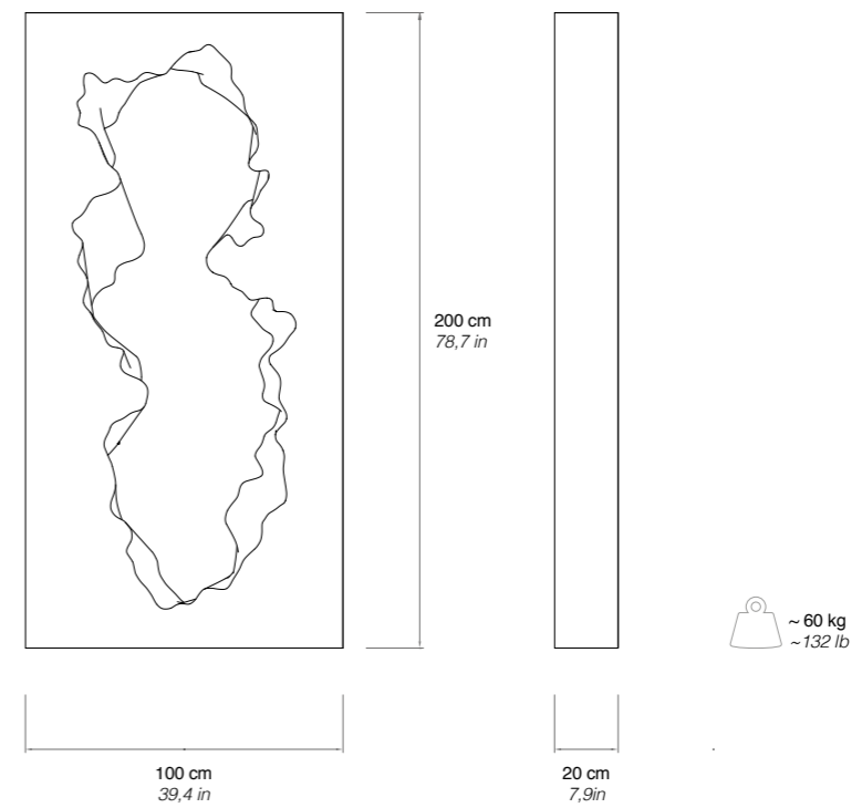
Mirror with frame in soft polyurethane hand finished with Guflac®.
